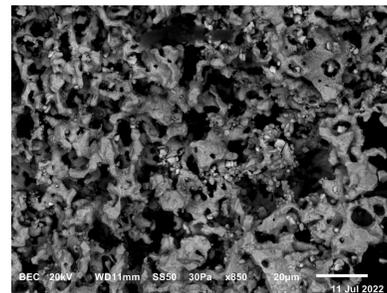
Figure 6: Post-etching SEM analysis shows a self-supporting network of Ni.
