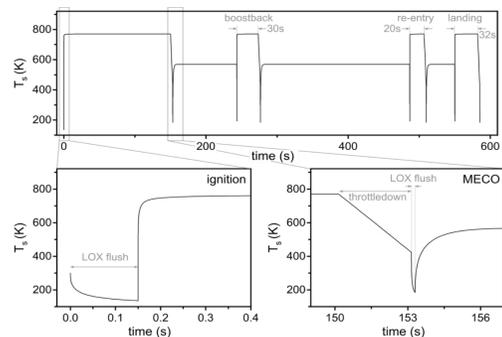
Figure 2: Predicted surface temperature of an EBC-coated surface in an ox-rich turbine of a reusable rocket engine during a single flight.
