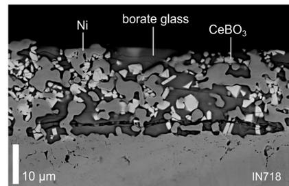
Figure 4: SEM image displaying the constituent materials of the EBC (10  $\mu\text{m}$  thickness).
