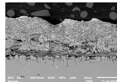
Figure 5: SEM image of IN718 sample after coating deposition (50  $\mu\text{m}$  thickness).
