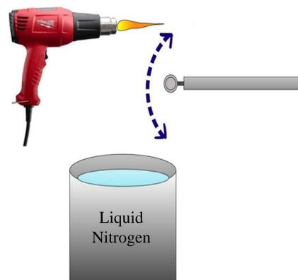
Figure 8: Schematic of the cyclic motion of the thermal shock rig between hot air gun and liquid nitrogen (LN).
