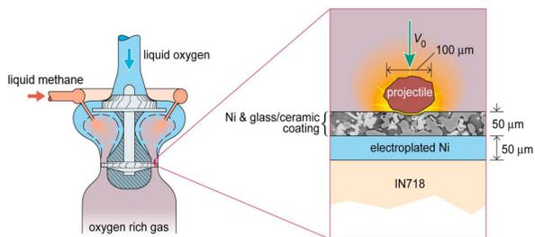
Figure 1: Schematic of an oxygen-rich turbopump assembly.
