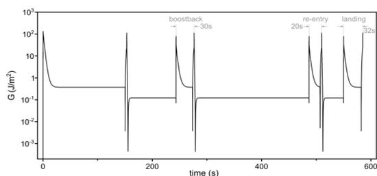
Figure 3: Strain energy release rate for the crack propagation at the interface of the ox-compatible coat and the nickel (Ni) coat during a single flight.
