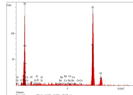
Figure 7: EDS analysis of the etched EBC pellet after using an Iron Chloride ( $\text{FeCl}_3$ ) solution.
